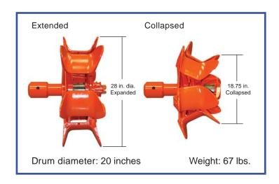
A half turn of the handle collapses the outer rim. The six rim segments pivot inward when the sliding spider is released allowing quick removal of wire or cable spool.
