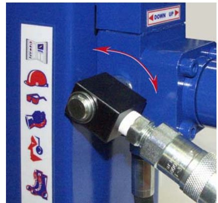
Swivel reduces hose strain and simplifies tool positioning .
