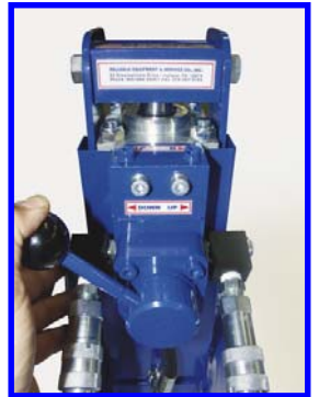
Move control valve into DOWN direction before inserting post or chain.
