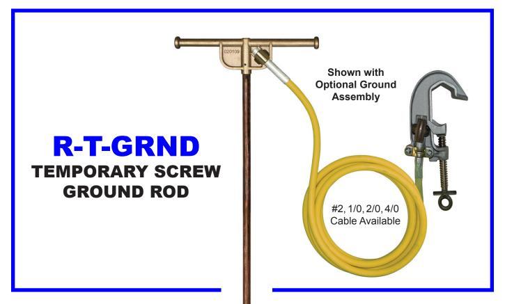
RELIABLE'S R-T-GRND Temporary Screw Ground Rod will provide a ground where a system ground is not available. When installed, the 6' spiraled ground rod developes less resistance than straight ground rods. (Actual resistance values depend upon soil properties)
