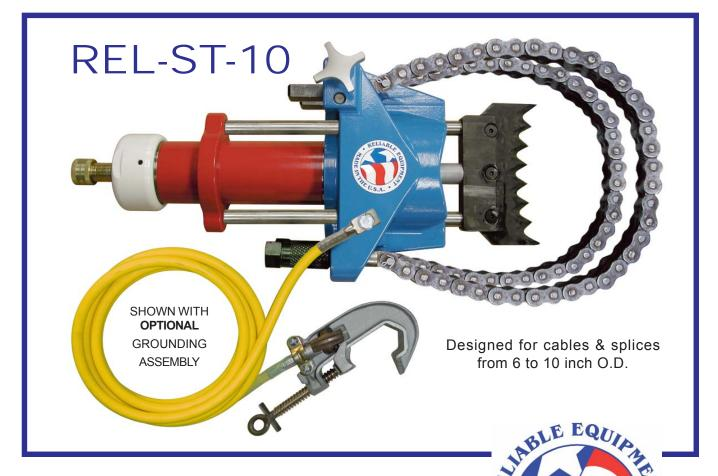
The REL-ST-10 double acting hydraulic spearing tool was designed to drive a serrated piercing blade into the conductor or joint ensuring that the conductor is out of service prior to beginning work.
